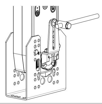
KH-AFB non-direct mounting with ZG-118 mounting bracket
