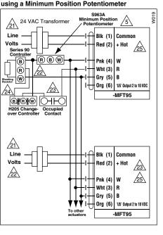
Wiring Multiple Actuators to a Series 90 Controller
