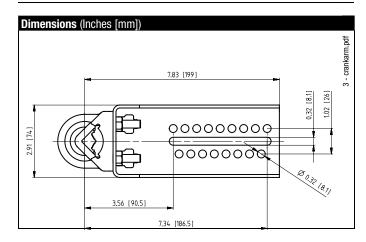
NOTE: The KH-EFB crank arm is designed to attach itself with the K9-2 clamp. The supplied rod must be used when the actuator is not direct coupled onto a shaft.
