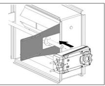
Mount directly to 1.05" jackshafts. (new ZG-120 bracket shown)
