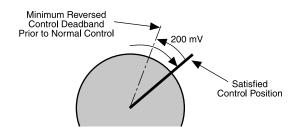
**Note:** Resolution is a percentage of operating range. 1% in one direction, 2.5% when changing direction. 2-10 VDC control example shown above.
