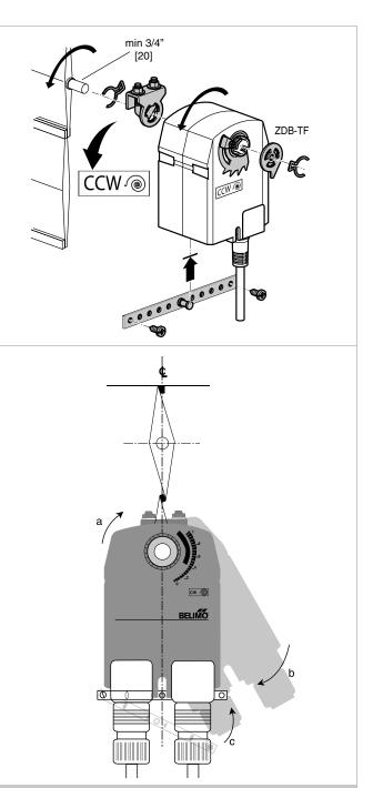
FIGURE D - Standard Mounting (Dimensions in Inches [mm])
