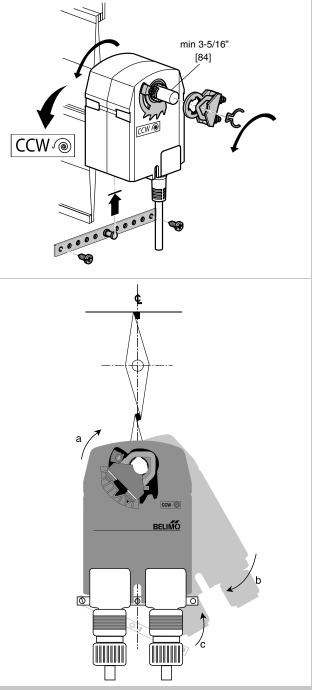
FIGURE B - Standard Mounting (Dimensions in Inches [mm])
